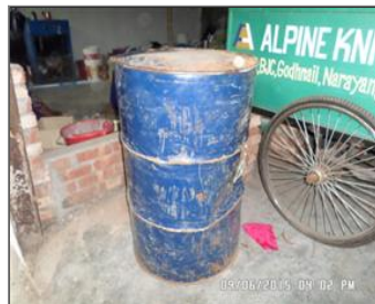
Photo of the inside of the main production hall NC B 11 4 4 No secondary containment.JPG
